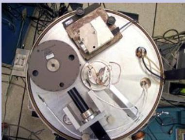
*A laser from the NIST-designed autocollimator (square device at top) is beamed at the mirrored polygon in the gray circle at left, and its reflection allows the angle of the polygon's faces to be precisely determined while the polygon rotates. The black device at bottom takes measurements that minimizes the wobbling the polygon experiences while spinning. Image: Hudson/NIST*
