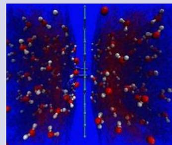
This is a figure showing the proton transfer channel across a quad-defect in graphene, as obtained from a ReaxFF molecular dynamics simulation. Image courtesy Murali Raju, Penn State.
