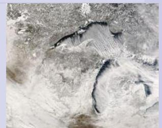
Cloud streets -- long rows of cumulus clouds oriented parallel to the direction of the wind -- are an everyday example of natural turbulent convection. Image courtesy MODIS
