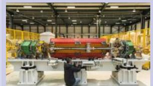
*An engineer tests the installation of a vacuum chamber for SESAME, at CERN's magnet-testing facility SM18. Credit: Maximilien Brice/CERN*
