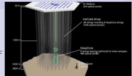
*IceCube is comprised of a cubic kilometer of ice, which is densely packed with optical modules. The detector is located deep below the surface – it starts 1½ km below the ice and ends at the bottom at a depth of 2½ km. The instruments in the detector are comprised of 86 cables each with 60 digital Optical Modules (extremely sensitive light sensors). Credit: IceCube Collaboration*
