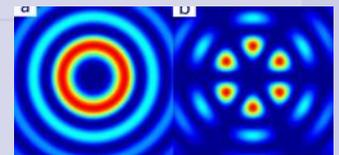
*By combining two structured light fields in the form of Bessel beams (a), the resulting beam of "petals" (b) spins as it travels. The spin can be made to speed up or slow down. Photos by Andrew Forbes.*
