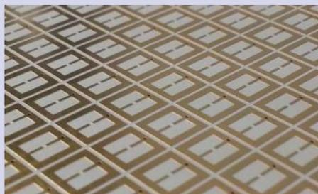
The metasurface used for collecting electromagnetic energy is shown. Credit: O.Ramabi/U.Waterloo
