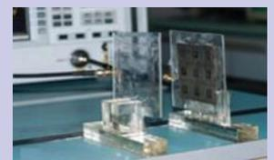
*Wireless power transfer between two coils. The metamaterial is the gray 3 x 3 square embedded into the coil on the right. Credit: Q. Wu, et al. ©2015 EPLA*
