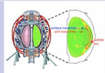
*Schematic of NSTX tokamak at PPPL with a cross-section showing perturbations of the plasma profiles caused by instabilities. Without instabilities, energetic particles would follow closed trajectories and stay confined inside the plasma (blue orbit). With instabilities, trajectories can be modified and some particles may eventually be pushed out of the plasma boundary and lost (red orbit). Image by Mario Podestà.*
