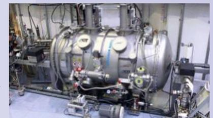
*SCU15 is a unique superconducting undulator for production of high-brilliance x-rays installed in the ANKA storage ring. Credit: KIT/ANKA/BNG*
