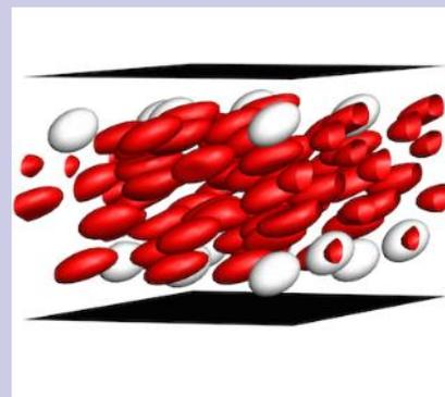
*An image from a simulation that shows a case in which the stiffer cells (white) are driven to the walls of a blood vessel. Mike Graham's paper lays out a new theory that predicts the conditions under which this process occurs.*
