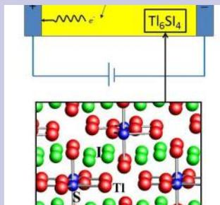
Schematic for a TI6SI4 detector and the crystal structure of TI6SI4. Credit: Mao-Hua Du/Oak Ridge National Laboratory, Oak Ridge, Tenn
