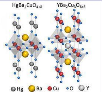
These are the crystal structures of  $HgBa_2CuO_{4+\delta}$  and  $YBa_2Cu_3O_{6+\delta}$ . Image courtesy Nature Communications.
