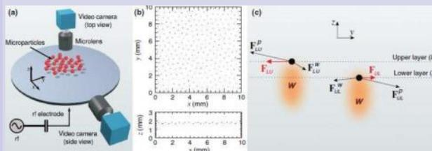
In the new experiments, two layers of microparticles levitating at two different heights above an electrode have allowed researchers to investigate the statistical mechanics of nonreciprocal interactions, which violate Newton's third law.
