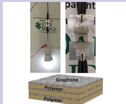
ORNL's ultrastrong graphene features layers of graphene and polymers and is an effective conductor of electricity. Image courtesy ORNL.
