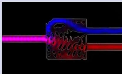
Infrared light enters this silicon structure from the left. The cut-out patterns, determined by an algorithm, route two different frequencies of this light into the pathways on the right. This is a greatly magnified image of a working device that is about the size of a speck of dust. Credit: Alexander Piggott
