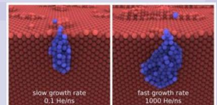
*Using their ParRep method on the Titan supercomputer, Los Alamos National Laboratory researchers were able to simulate the surface morphology for helium bubbles growing inside of a fusion reactor's divertor wall for two different growth stages. The combination of Titan and the ParRep method completed simulations in 30 minutes that would have taken months using traditional molecular dynamics approaches. Credit: Luis Sandoval, Arthur Voter, Blas Uberuaga, and Danny Perez*
