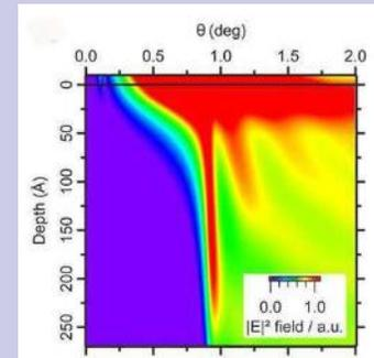
*A new X-ray based technique for studying buried interfaces reveals that the more the incident angle increases, the deeper the X-rays penetrate the system, allowing for depth-resolved analysis of the system.*
