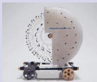
Eva, the first evaporation-powered car, rolls along, thanks to a moisture mill - a turbine engine driven by water evaporating from wet paper strips lining its walls. Eva is one of the many devices created to harness evaporation energy. Image courtesy Sabina Laboratory, Columbia University.
