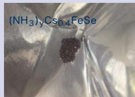
Figure 1. The  $(NH_3)_yCs_{0.4}FeSe$  sample prepared by liquid ammonia technique.
