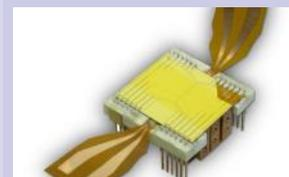
*The atom chip used to control the atoms. Credit: TU Wien*
