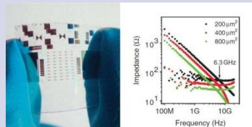
*(Left) Photograph of the flexible IGZO Schottky diodes. (Right) The highest frequency achieved by the flexible diodes is 6.3 GHz, which can accommodate all transmission frequencies of wireless communication. Credit: Zhang, et al. ©2015 Macmillan Publishers Limited*
