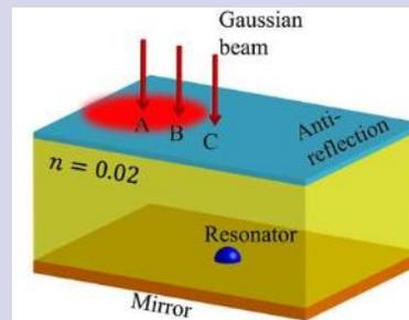
*A diagram shows an optical nanoresonator embedded within a slab of low-index material to test its performance.*
