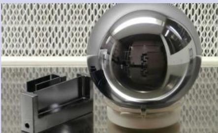
*The number of atoms in this silicon sphere is known given or taken 20 atoms each  $10^9$ . The atom distance was measured by the X-ray interferometer on the left. Credit: Enrico Massa and Carlo Sasso*
