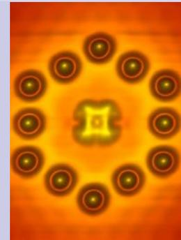
Scanning tunneling microscope image of a phthalocyanine molecule centered within a hexagon assembled from twelve indium atoms on an indium arsenide surface. The positively charged atoms provide the electrostatic gate .....
