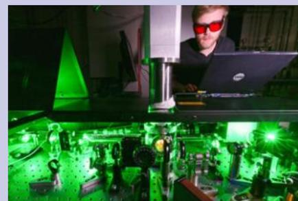
*This the 2-D ultra-fast UV spectroscopy set-up at EPFL's Laboratory of Ultrafast Spectroscopy, used to carry out the measurements in this study. Photo: Alain Herzog/EPFL*
