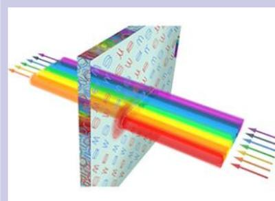
*An array of helical elements absorbs radiation of a certain frequency while casting no shadow in light over a range of other frequencies.*
