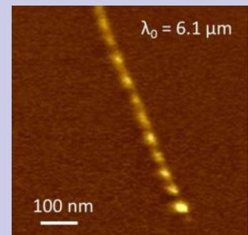
This s-SNOM infrared image shows Luttinger-liquid plasmons in a metallic single-walled nanotube. Credit: Courtesy of Feng Wang, Berkeley Lab
