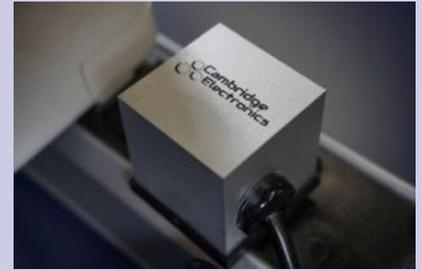
Shown here is a prototype laptop power adapter made by Cambridge Electronics using GaN transistors. At 1.5 cubic inches in diameter, this is the smallest laptop power adapter ever made. Image: Cambridge Electronics
