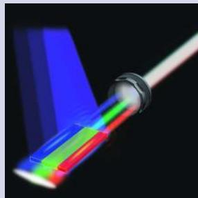
This schematic illustrates the novel nanosheet with three parallel segments created by the researchers, each supporting laser action in one of three elementary colors. The device is capable of lasing in any visible color, completely tunable from red, green to blue, or any color in between. When the total field is collected, a white color emerges.
