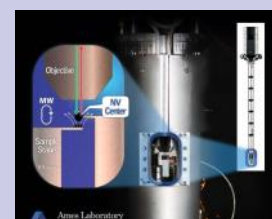
Physicists at the U.S. Department of Energy's Ames Laboratory are using an NV-magnetometer to make use of nitrogen-vacancy centers in diamond to sense extremely weak magnetic fields in nano- and mesoscale magnetic materials.
