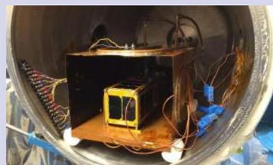
A thermal vacuum test of the Low Mass Radio Science Transponder-Satellite (LMRST-Sat) was performed at California Polytechnic State University, San Luis Obispo, California, in February of this year. The six-hour test, carried out in a partial vacuum....
