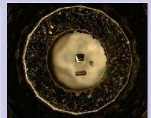
One of the metallic samples studied, niobium diselenide, is seen here - the square in the center-as prepared for an X-ray diffraction experiment. Image courtesy University of Chicago/ Argonne National Laboratory.
