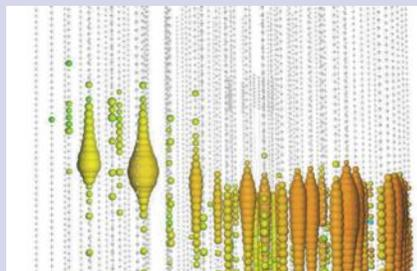
*An IceCube event display showing the latest 'most energetic event.' Each open circle is an un-hit optical module; the filled spheres show hit modules, with the radius indicating the number of detected photons. The colors indicate the relative time (red is first, then orange, yellow, green, and blue), but with the chosen scale, the timing isn't that useful. Credit: Leif Radel*
