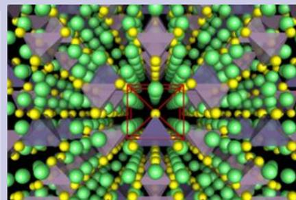
Illustrations show the crystal structure of a superionic conductor. The backbone of the material is a body-centred cubic-like arrangement of sulphur anions. Lithium atoms are depicted in green, sulfur atoms in yellow, PS4 tetrahedra in purple, and GeS4 tetrahedra in blue. Researchers have revealed the fundamental relationship between anion packing and ionic transport in fast lithium-conducting materials. Image: Yan Wang
