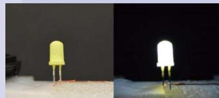
An LED coated with a yellow "phosphor" is shown turned off (left) and then turned on (right). This "green" LED is inexpensive and provides warm white light. Credit: Zhichao Hu, Ph.D.
