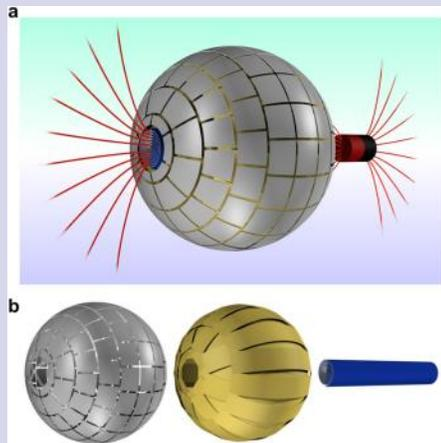
(a) The field of a magnetic source (right) is appearing as an isolated magnetic monopole when passing through the magnetostatic wormhole; the whole spherical device is magnetically undetectable. (b) The wormhole is composed of (from left to right) an outer spherical ferromagnetic metasurface, a spherical superconducting layer, and an inner spirally wound ferromagnetic sheet. Credit: Scientific Reports 5, Article number: 12488 (2015) doi:10.1038/srep12488
