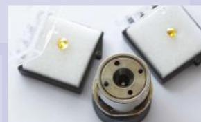
The apparatus the team led by Mikhail Erements at the Max Planck Institute for Chemistry in Mainz uses to generate extremely high pressures, is amazingly handy. The researchers press the metal cell with Allen screws together. The high pressure thus created in the center of the cell, only diamonds resist. The gems operate like anvils that compress a sample. Credit: Thomas Hartmann
