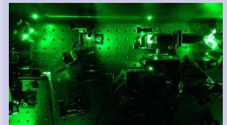
An image from an experiment in the quantum optics laboratory in Cambridge. Laser light was used to excite individual tiny, artificially constructed atoms known as quantum dots, to create "squeezed" single photons. Credit: Mete Atature
