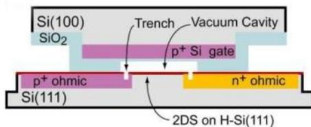
The upper half of the structure (using a different kind of silicon, Si100), constitutes the gate. Beneath the gate (the white region) is a small vacuum cavity. Directly beneath the vacuum region is the slab of silicon (111) material. The very topmost layer is impregnated with hydrogen atoms (H) is the crucial real estate. This layer supports a 2-dimensional electron system (2DES) of charges running between the source and the drain.
