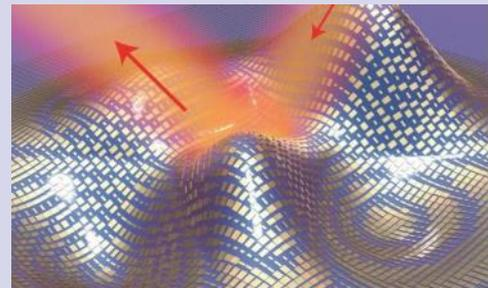
*A 3-D illustration of a metasurface skin cloak made from an ultrathin layer of nanoantennas (gold blocks) covering an arbitrarily shaped object. Light reflects off the cloak (red arrows) as if it were reflecting off a flat mirror. Credit: Xiang Zhang group, Berkeley Lab/UC Berkeley*
