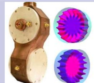
(Left) Photo of the orthogonal sapphire crystal mount, with (right) simulations of the electromagnetic resonant mode patterns. A frequency variation in the resonance would indicate a variation in the speed of light. Credit: Stephen R.
