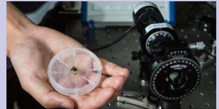
The circularly polarized light detector on a chip, on the left, performs the same function as the conventional, optically based detector on the right. Credit: Anne Rayner, Vanderbilt University
