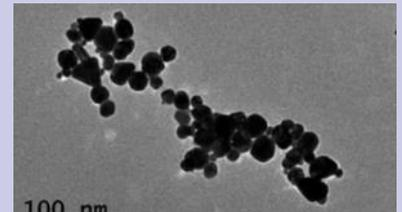
*Microscopic view of microplasma-gold nanoparticles on a new, highly sensitive, test strip that enables early detection of heart attacks.*
