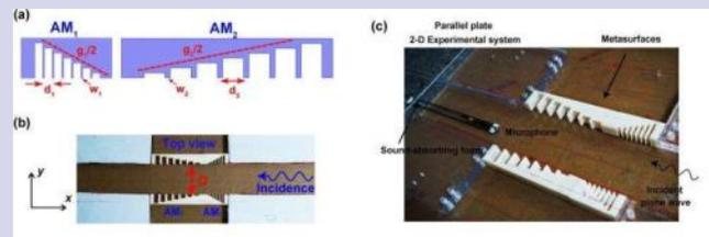
(a) The two acoustic metamaterials have different groove patterns, which are positioned at different sides of the tunnel so that they affect the sound waves differently depending on which direction they're coming from. (b) and (c) Photographs of the open tunnel. Credit: Zhu, et al. ©2015 AIP Publishing
