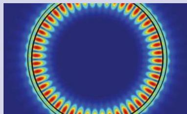
*In the whispering gallery mode of a 2-D excitonic laser made from a monolayer of tungsten disulfide and a microdisk resonator, the localization of the electric field at the edges of the resonator helps promote a high Q factor with low power consumption. Credit: Xiang Zhang, Berkeley Lab*
