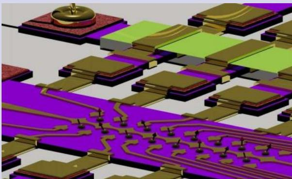
3D artist impression of a large array of quantum devices in which charge is "locked" onto the electrodes, which allows each wire to act like multiple wires. Credit: R. K. Puddy, University of Cambridge
