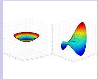
*A rotationally symmetric optic is traditionally used in telescopes. The freeform optic on the right takes a different shape and is now being investigated for use in space-based instruments. Image courtesy NASA.*
