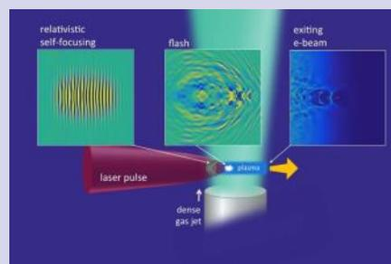
*This schematic illustrates the laser-driven electron accelerator experiment at the University of Maryland.*
