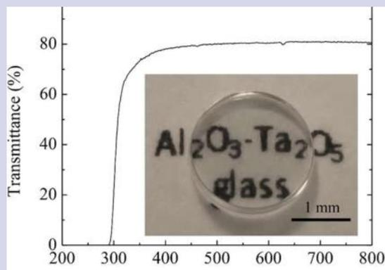
Transmittance spectrum of the  $54Al_2O_3-46Ta_2O_5$  glass in the UV/vis region. The inset picture shows the glass sample used for the transmittance experiment. Credit: (c) 2015 *Scientific Reports* (2015). DOI: 10.1038/srep15233
