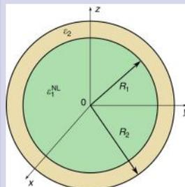
*The optical meta-atom has a core (with radius  $R_1$ ) and shell (with radius  $R_2$ ). Light of a specific wavelength (quantized energy) can be trapped inside the core. Credit: Lannebère, et al. CC-BY-4.0*
