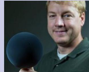
Principal Investigator Phillip Chamberlin holds a sphere coated in super-black carbon nanotubes. Image courtesy NASA/W. Hrybyk.
