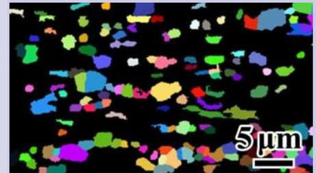
By creating a patchwork of large, soft-grained columns (shown here in multiple colors) in a harder, ultrafine-grained matrix (shown here in black), researchers have found a way to increase metal strength without sacrificing ductility. Credit: Yuntian Zhu, North Carolina State University
