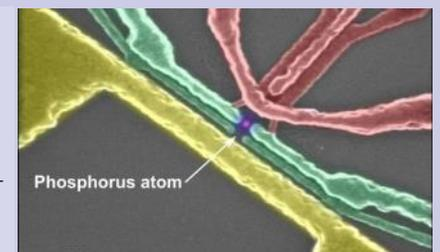
False-colour electron microscope image of the silicon nanoelectronic device which contains the phosphorus atom used for the demonstration of quantum entanglement. Credit: University of New South Wales
