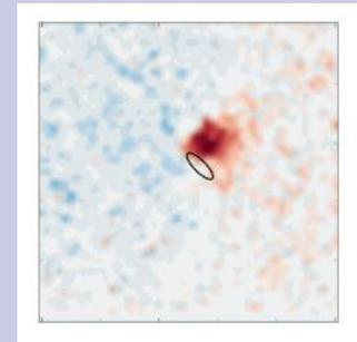
An ultrafast camera coupled to a custom-built X-ray microscope at SLAC's Stanford Synchrotron Radiation Lightsource allowed researchers to produce a six-frame "movie" of the soliton's motion. It took about 12 hours to record enough X-ray data to produce the movie. Credit: Stefano Bonetti/Stockholm University
