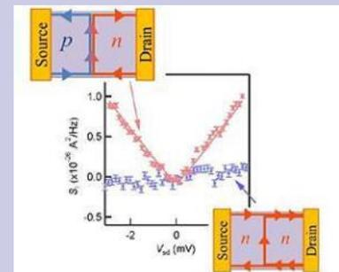
This is the result of the shot noise measured in our device. Non-zero shot noise due to the electron partition process is observed in the p-n junction case (red dots). On the other hand, there appears no noise in the unipolar regime (blue dots). Image courtesy Osaka University.
