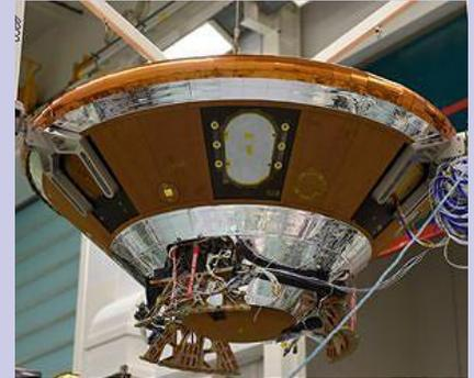
*Schiaparelli, also known as the ExoMars Entry, descent and landing Demonstrator Module is seen here being installed at the top of the Trace Gas Orbiter, at Thales Alenia Space, in Cannes, France, on 25 November 2015. The first mission of the ExoMars programme, scheduled to arrive at Mars in 2016, consists of a Trace Gas Orbiter plus an Entry, Descent and Landing Demonstrator Module (EDM).*
