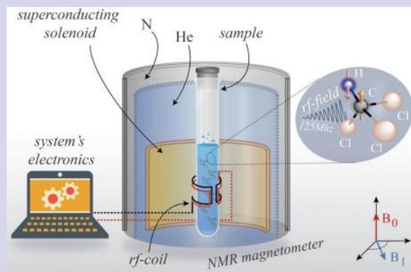
In the experiment, a sample of liquid chloroform ( $\text{CHCl}_3$ ) is placed at the center of a superconducting magnet inside a nuclear magnetic resonance (NMR) magnetometer. Forward and reverse magnetic pulses are applied to the sample, which drives the carbon nuclear spins out of equilibrium and produces irreversible entropy. Credit: Batalhão, et al. ©2015 American Physical Society
