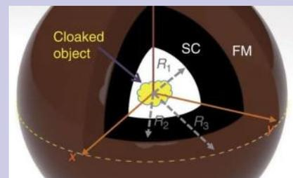
The bilayer cloak consists of an inner superconducting shell and an outer ferromagnetic shell, whose opposite effects on an external magnetic field completely cancel each other out to shield a cloaked magnetic object (yellow) from the external magnetic field. Credit: Zhu, et al. ©2015 *Nature Communications*
