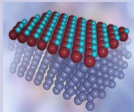
This is a computer visualization of a single layer of a new form of iron oxide on a platinum substrate. Iron atoms in brown, oxygen atoms in light blue. Image courtesy IFJ PAN.
