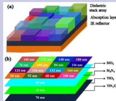
(a) Schematic diagram of monolithic integrated colored solar selective absorber array with structure of IR reflector/absorption layer/dielectric stack. (b) Schematic diagram of monolithic integrated colored solar selective absorber array with different thickness of SiO<sub>2</sub>. Credit: *Optics Express*
