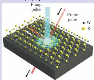
Researchers at the Gedik Lab at MIT use strong ultrafast laser pulses to stimulate changes in material, followed by a weaker probe laser pulse after some time delay to monitor the changes with femtosecond time resolution. Tungsten (W) atoms are black, and sulfur (S) atoms are yellow. Credit: Edbert Jarvis Sie
