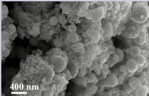
*A femtosecond laser created detailed hierarchical structures in the metals, as shown in this SEM image of the platinum surface. Image: The Guo Lab/Univ. of Rochester*
