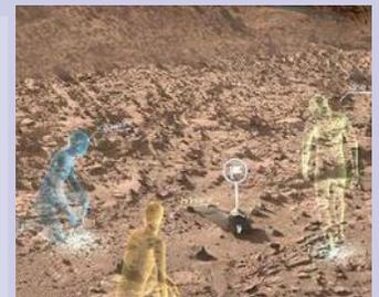
*New NASA software called OnSight will use holographic computing to overlay visual information and data from the agency's Mars Curiosity Rover into the user's field of view. Holographic computing blends a view of the physical world with computer-generated imagery to create a hybrid of real and virtual. Image courtesy NASA.*
