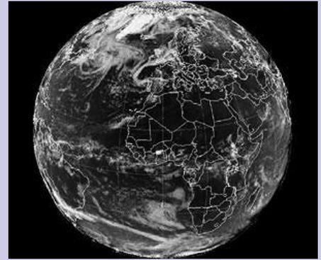
The 10 wavelengths captured by NASA's Earth Polychromatic Imaging Camera provide data on Earth's surface and atmosphere. The 388 nanometer UV channel here allows scientists to study the energy reflected by ice sheets and clouds, an important measurement in climate studies. Image courtesy NASA.
