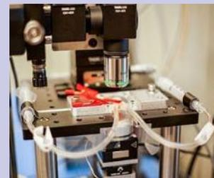
A new high-speed microscope produces images of chemical processes taking place at the nanoscale, at a rate that is close to real-time video. This closeup shot of the microscope shows transparent tubes used to inject various liquids into the imaging environment. This liquid can be water, acid, buffer solution for live bacteria, cells, or ...
