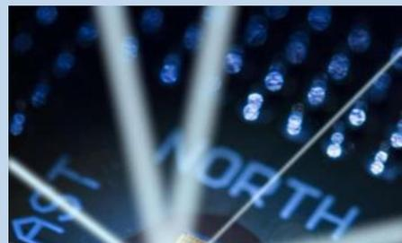
*This packaged electronic-photonic processor microchip under illumination reveals the chip's primary features. The light rays emanating from the chip are drawn to show that the processor talks to the outside world using light. Credit: Glenn J. Asakawa, University of Colorado*
