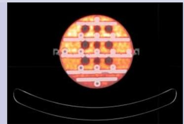
*A fused PET-CT image of the new phantom with its traceably calibrated amount of fluorine-18 (orange). The circular objects are the MR-visible test spheres; in this PET-CT image they appear as regions with no PET response.*
