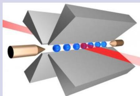
An ion trap of the type used in the experiment. Credit: Institute of Theoretical Physics, Innsbruck
