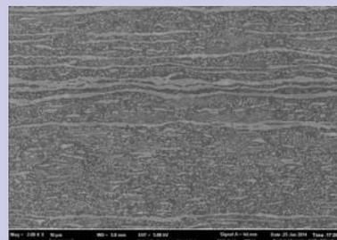
Annealed microstructure of high-specific-strength steel (HSSS). Fine FeAl-type B2 precipitates form during annealing in between the B2 stringer bands in steel matrix. The specimen was annealed for 15 min at 900C. Credit: Hansoo Kim
