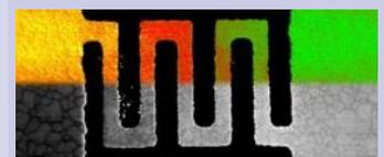
This composite image shows density (grey) and temperature (color) maps of a 100 nm-wide polycrystalline aluminum wire. The temperature is computed from the density using aluminum's known thermal expansion. Lower densities appear at crystal-grain boundaries, which are atomic-scale features, and where thermal expansion has caused the aluminum to expand. One end of the wire (green) is near room temperature, and the other (orange) is 160 K warmer. Credit: USC CEMMA & UCLA Regan
