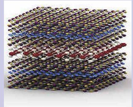
LED Heterostructure Schematic.
