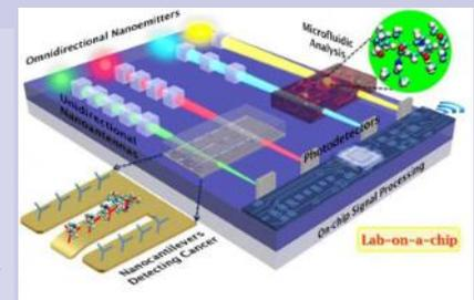
*This is a schematic representation of unidirectional cubic nanoantennas inducing directionality to omnidirectional nanoemitters (light sources, e.g., spasers, quantum dots), to precisely focus light with adjustable beam width and intensity, which can be tuned by adjusting the length of nanocube chain or intercube spacing. ...*
