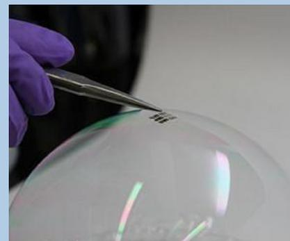
The MIT team has achieved the thinnest and lightest complete solar cells ever made, they say. To demonstrate just how thin and lightweight the cells are, the researchers draped a working cell on top of a soap bubble, without popping the bubble. Image courtesy Joel Jean and Anna Osherov.
