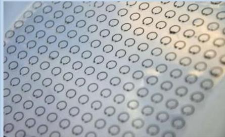
*This flexible, stretchable and tunable "meta-skin" can trap radar waves and cloak objects from detection. Credit: Liang Dong/Iowa State University*
