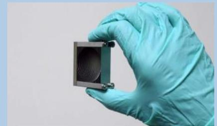
Researchers have used an array of stacked plates to make a lens for terahertz radiation. The technique could set stage for new types of components for manipulating terahertz waves. Credit: Mittleman lab / Brown University
