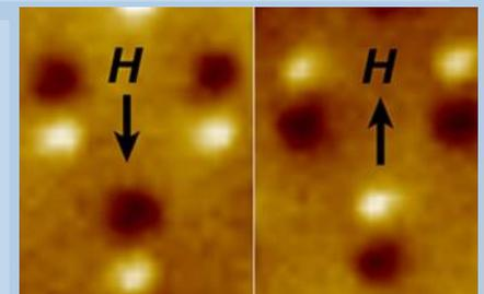
Magnetic microscope image of three nanomagnetic computer bits. Each bit is a tiny bar magnet only 90 nanometers long. The microscope shows a bright spot at the "North" end and a dark spot at the "South" end of the magnet. The "H" arrow shows the direction of magnetic field applied to switch the direction of the magnets. Credit: Jeongmin Hong and Jeffrey Bokor
