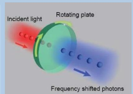
For a circularly polarized pumping laser passing through the nonlinear optical crystal along its rotation axis, second harmonic generation with opposite spin state has a frequency shifts of  $\pm 3\Omega$ . Credit: University of Birmingham
