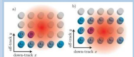
Illustration of two versions of the HAMR writing procedure, showing a laser being used to heat bit B, which enables the bit to be written by a much smaller magnetic field than would otherwise be required. All of the surrounding A bits remain in their original states because they have not been heated (enough), and so cannot be written by the magnetic field. Credit: Vogler, et al. ©2016 AIP Publishing
