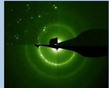
*This is a transmission electron microscopy image of different levels of crystallinity in the amorphous alloy. Image courtesy Jacobs School of Engineering/UC San Diego.*
