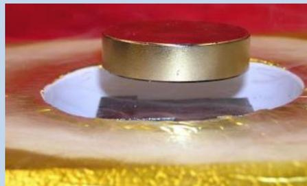
This image of a magnet levitated over a high-temperature superconductor array shows rectangular TFMs (black) levitating a heavy ferromagnet (silver) above a container of liquid nitrogen. Credit: Weinstein/University of Houston
