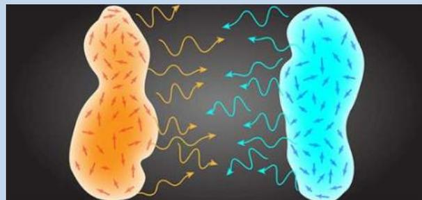
*Two bodies at different temperatures in vacuum constantly exchange heat. This energy flux is mediated by photons (shown here as wavy lines), which are generated by thermally fluctuating electrical currents (arrows) inside each body.*
