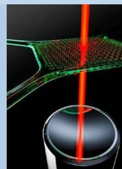
*An artist's impression of the membrane coupled to a laser beam. The periodic pattern makes the device highly reflective, while the thin tethers allow for ultra-low mechanical dissipation. Credit: Felix Fricke*
