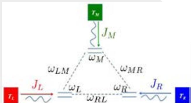
The quantum thermal transistor consists of three two-level systems, which can be implemented as spins with an up and a down state. Any one of these systems can control the heat current that flows to the other two, resulting in switching their spins. Credit: Joulain et al. ©2016 American Physical Society
