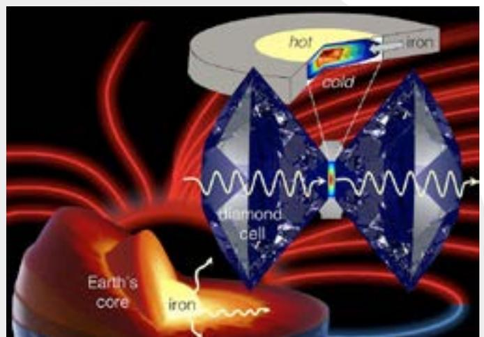
*Illustration of how the diamond anvil cell is used to mimic and study planetary core conditions. Credit: Stewart McWilliams*
