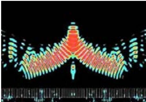
Light passing through the metalens is focused by the array of nanostructures on its surface. Image courtesy Capasso Lab/ Harvard John A. Paulson School of Engineering and Applied Sciences.
