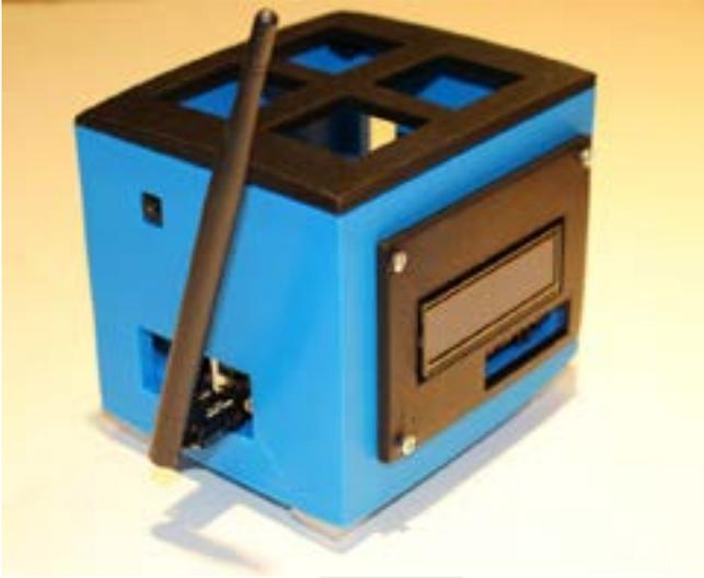
*Pi-Sat is a small satellite based on the Raspberry Pi computer. It is low-cost and easy to use, making it ideal for classroom-built satellites. Image courtesy NASA/Alan Cudmore.*
