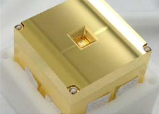
Test masses carved from blocks of high purity gold-platinum alloy, and weighing nearly 2 kilograms, are flying aboard the LISA Pathfinder spacecraft in the development of systems that will detect gravitational waves as part of the forthcoming LISA space-based gravitational wave observatory. Credit: European Space Agency, CGS SpA
