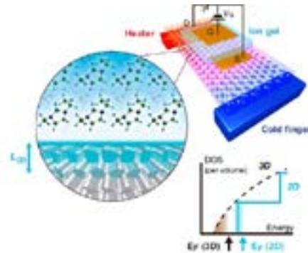
The enlarged illustration (in the circle) shows a 2D electron gas on the surface of a zinc oxide semiconductor. When exposed to a temperature difference, the 2D region exhibits a significantly higher thermoelectric performance compared to that of bulk zinc oxide. The bottom figure shows that the electronic density of states distribution is quantized for 2D and continuous for 3D materials. Credit: Shimizu et al. ©2016 PNAS
