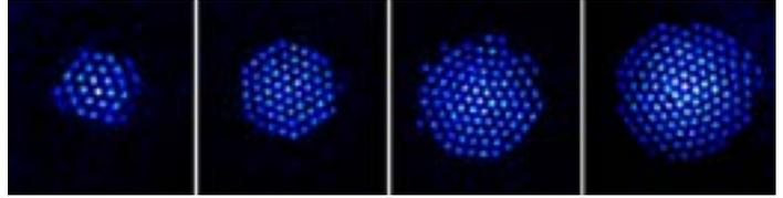
NIST physicists have built a quantum simulator made of trapped beryllium ions (charged atoms) that are proven to be entangled, a quantum phenomenon linking the properties of all the particles. The spinning crystal, about 1 millimeter wide, can contain anywhere from 20 to several hundred ions. Credit: NIST
