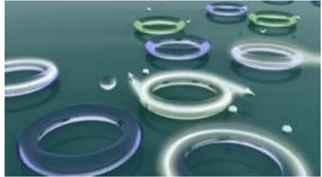
Artist's view showing the control of the emission direction of lasing at exceptional points in a whispering gallery mode micro-laser. The tori and the spheres represent the microtoroid resonators and the scatterers, respectively. With two scatterers with appropriate sizes and locations in the field of the resonator, light is emitted in only one direction. The lasing is bidirectional when there is one or no scatterer. Credit: B. Peng, F. Monifi, S. K. Ozdemir and L. Yang
