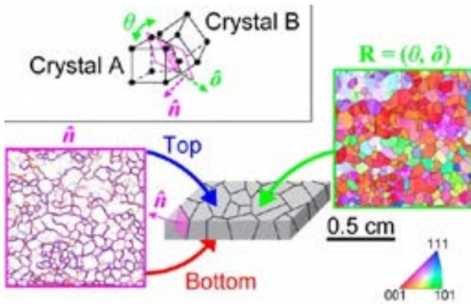
The method combines optical microscopy techniques (left, in pink) with electron backscatter diffraction (right, in green) to measure characteristics of the boundaries between crystal grains, which help determine the material's overall properties. Credit: Matteo Seita
