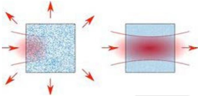
Materials made of a large number of particles placed at random in a homogeneous medium will strongly scatter light, and thus no transmitted beam emerges (left). However, a hyperuniform material made of the same particles at the same density will appear transparent because scattering is suppressed, and the incident beam of light is transmitted (right). Credit: Rémi Carminati, Romain Pierrat, Institut Langevin, ESPCI Paris, CNRS
