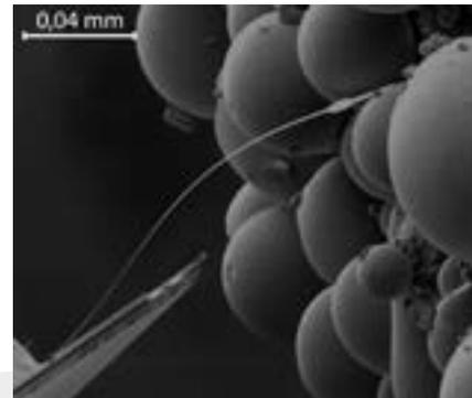
NMR microscope, consisting of a thin wire and a small magnetic ball (fake colour purple). The purple ball induces a uniform magnetic field, so that the surrounding atomic nuclei all line up with their axis pointing in the same direction. The researchers send radio waves through their sample, causing some nuclei to flip the other way, and measure how long it takes before they flip back again. Credit: Leiden Institute of Physics
