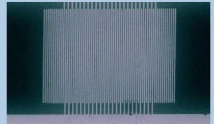
A colorized micrograph of a NIST single-photon detector made of superconducting nanowires patterned on molybdenum silicide. Credit: Verma/NIST
