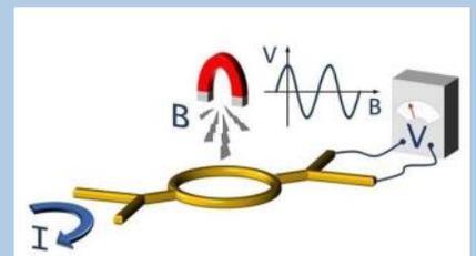
Schematic representation of the nonlocal electron interference experiment. A dc current is driven from the upper left to the lower left contact. A nonlocal, oscillating voltage is measured between the upper and lower right contacts due the magnetic-field induced single-electron interference in the 500 nanometer ring in the middle.
