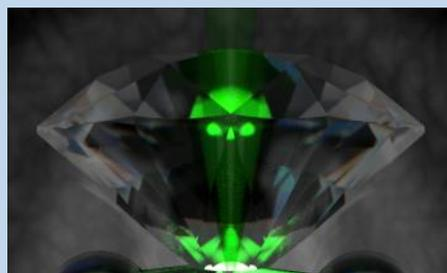
*An artistic representation of a hydrogen molecule under compression using opposed diamond anvil devices. The experimental work using micro-focused Raman spectroscopy explores the possibility of breaking the hydrogen molecule through means of room-temperature compression in an attempt to reach the long proposed metallic state of hydrogen. Credit: Philip Dalladay-Simpson and Eugene Gregoryanz*
