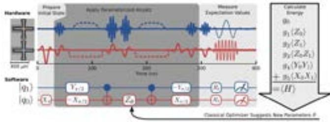
Hardware and software schematic of the variational quantum eigensolver. Credit: Physical Review X (2016). DOI: 10.1103/PhysRevX.6.031007
