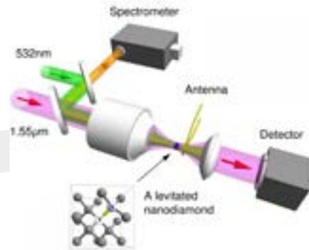
A schematic of an optical tweezer used in a vacuum chamber by Purdue University researchers, who controlled the “electron spin” of a levitated nanodiamond. The advance could find applications in quantum information processing, sensors and studies into the fundamental physics of quantum mechanics. (Purdue University image/ Tongcang Li)
