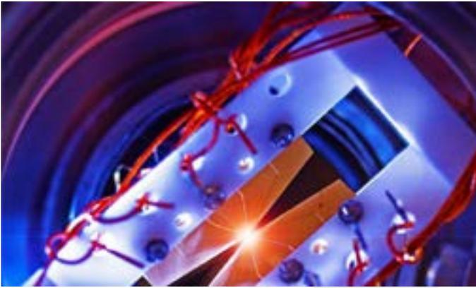
An ion trap with four segmented blade electrodes used to trap a linear chain of atomic ions for quantum information processing. Each ion is addressed optically for individual control and readout using the high optical access of the trap. Credit: Emily Edwards
