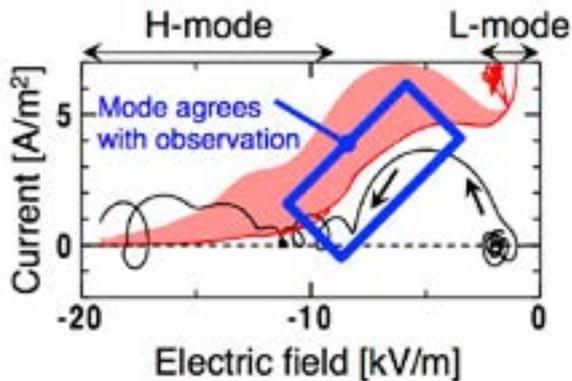
The right side of the figure where the electric field's absolute value is small corresponds to the L-mode plasma and the left side having large electric field to the H-mode. The black line indicates the experimental value of the electric current and the red line the theoretical value used in the model based upon differences in the trajectories. Credit: Tatsuya Kobayashi
